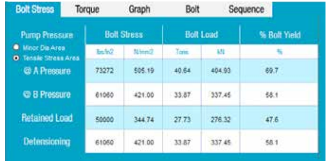
Bolt Stress window, displays bolt stress, bolt load and % of bolt yield.
